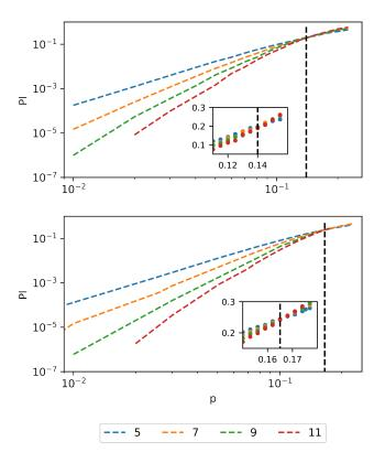
FIG. 5: Logical error rate as a function of the physical qubit error rate of the symmetric depolarizing channel for four different distance rotated planar codes. The top figure shows the results for the conventional MWPM decoding method. The bottom figure portrays the results for the recursive MWPM method. The black dashed lines indicate the location of the threshold.
