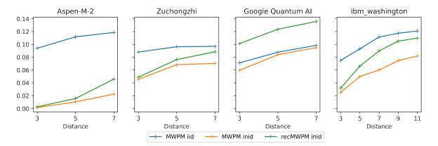
FIG. 7: Probability pseudo-thresholds as functions of the code distances for four different sets of qubits under three different scenarios. The blue curves consider i.i.d. conditions and are decoded through MWPM. The orange and green curves consider i.ni.d. noise decoded with MWPM and recMWPM, respectively.
