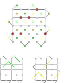
FIG. 2: Decoding of a  $5 \times 5$  rotated planar code via minimum weight perfect matching. On the top, the rotated planar code experiences an error, the non-trivial Pauli operators on the data qubits are represented through red circles. Measurement qubits which experience a change in measurement due to the error are denoted in light green and light yellow circles with an exclamation mark. On the bottom, the X-check and Z-check subgraphs with the resulting MWPM computation are shown.
